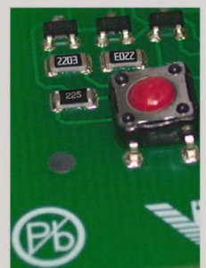
Micro Switch surchauffé
